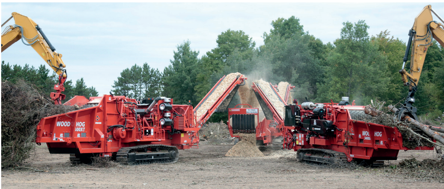
This year’s Morbark Demo Days culminated with demonstrations of equipment for the forestry, biomass, recycling, and tree care markets that ended with a 3400 XT and 6400 XT Wood Hog tracked horizontal grinders feeding into another 6400 XT Wood Hog for regrinding (photo Morbark).
