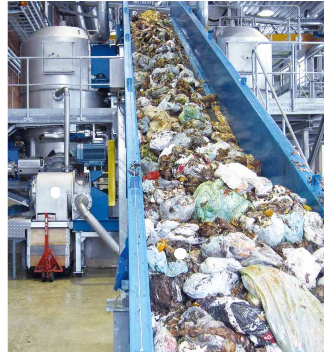
Household waste may not look pretty or smell nice but it has an energy and material recovery value. Separating the two is the challenge even if it arrives at a plant source separated. Here the RTC 1-tonne-per-hour pre-treatment unit testing a batch of client feedstock with (1) infeed from the receiving bin to the (2) HC-pulper. (3) the reject separator (photo courtesy Cellwood Machinery).
