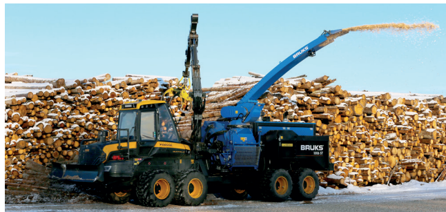
A Bruks 1006 ST chipper mounted on a Ponsse Buffalo forwarder making short work of fuelwood at a biomass terminal in Sweden.
